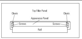
Place rail against cleats and flush with the outside edges of the cleats. Secure with wood screws. If the appearance panel is very narrow, cleats can be attached to the rail.
